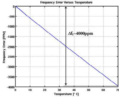
Figure 1. Temperature dependence of an LC-tank resonance frequency.
