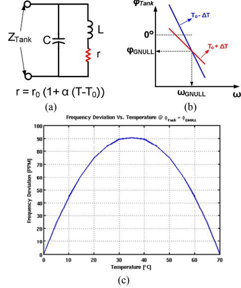
Figure 5. (a) Simple first order model of an LC-tank, (b) Global Null of an LC-tank and (c) Frequency deviation at GNULL phase.
