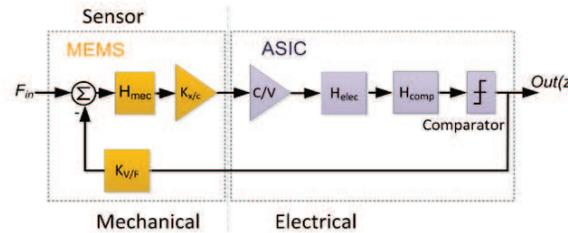
Fig. 2:  $\Sigma$ - $\Delta$  based closed-loop sensor.
